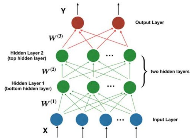
**FIGURE 1** Deep neural network (DNN) structure
